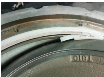
Radiation caused damage of seals of valves
