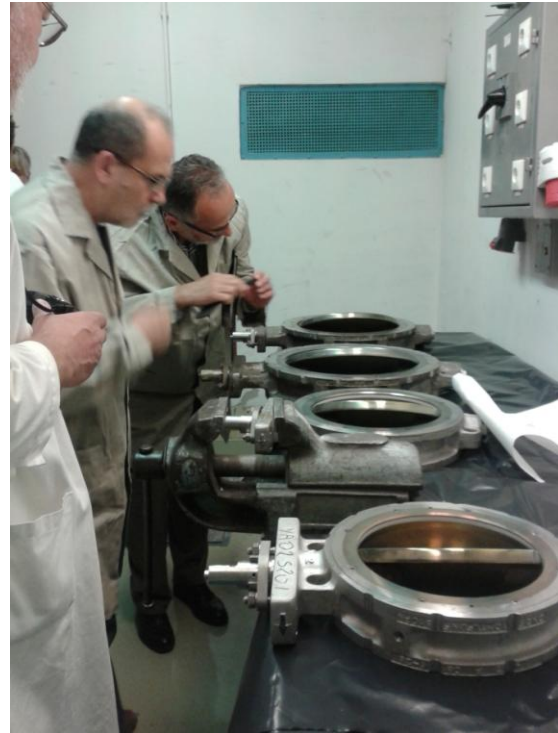
The regulatory inspection of damaged seals
